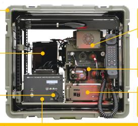
The radio equipments are quickly removable. RFDS unit can be supplied without radio equipment so that Barrett customers can use their wisting aguipment.
