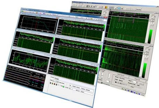
The UASA performs Low Frequency (LOFAR) Sonar data collection, processing, analysis, classification and database management. The LOFAR data, which consists of acoustic signals radiated by various sources, is received and collected by naval and air platforms operating passive sonar systems such as submarines, surface platforms with towed arrays, air platforms using sonobuoys, fixed bottom-moored sonar systems, etc.
