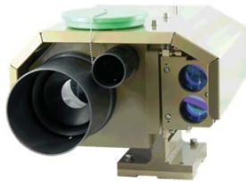
Optoelectronics box with Laser Range Finder
