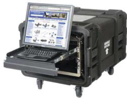
Figure 7 | Ruggedized Laptop configuration for rack case
