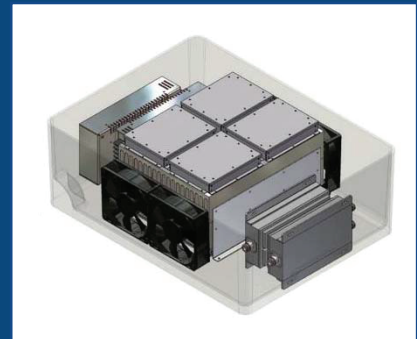
Figure 3 System installation in the rugged briefcase with independent power supply, battery, receiver, PA module and cooling system.
