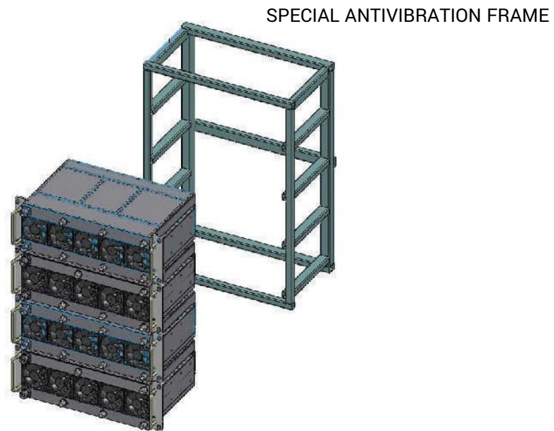
JAMMING SYSTEM MODULES
