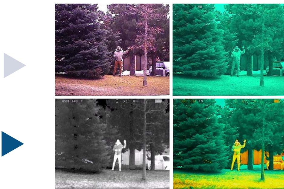
What differentiates the TB-QUAD4 is that with the fusion mode you are never left in pitch darkness. All channels complement each other to produce real-time, no-lag video images and unmatched situation awareness. This is achieved by combining detailed images from the visible/near infrared and long-wave infrared spectrum ranges. The end result is a tactical binocular with superb detection and recognition capabilities.
