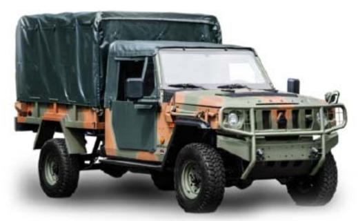
C4I-AM21 - ¾ Ton, is a vehicle for transporting personnel or cargo of 750 kg. It has a hood, metal body and cabin with a canvas roof. Its strong and robust power train, the wide suspension travel and the resistance of the assembly, make this model an ideal utility to carry out military tasks in the most difficult terrain. Also available in RHD version (right hand drive)
