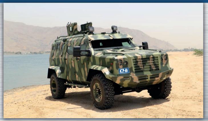
Full vehicle armoring with certified ballistic material up to CEN B7/ NIJ IV/ .50cal, including front, sides, rear, roof and floor, designed to resist incoming ballistic threats from any angle. The Guardian features a special light weight armor package designed to minimize the curb weight and maximize mobility and off-road capability.
