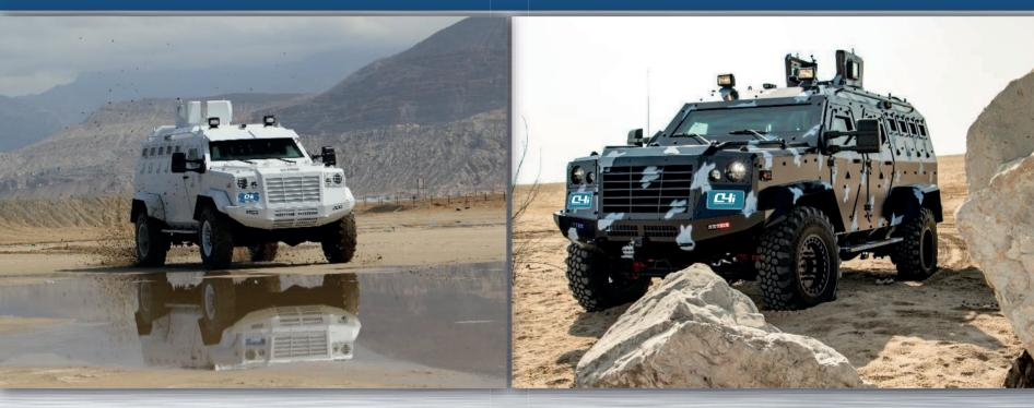
Based on the Ford F550 Super Duty chassis, the C4i guardian is an armored personnel carrier that provides high level of ballistic and blast resistance. Upgraded components to the suspension and drive train maximize the off-road abilities of the vehicle while providing a smooth on-road ride.
