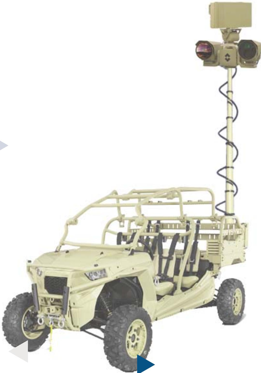
The C4I-LTV Light Tactical Vehicle is a lightweight all terrain reconnaissance and surveillance system that features a 4-passenger design. Quickly deployable, C4I-LTV gives operators the ability to go almost anywhere and conduct fully self-contained surveillance missions using advanced radar, electro-optical, and thermal imaging systems.
