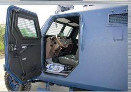
Full Vehicle armoring with certified CEN B6/NIJ III Level ballistic material, including front, sides, rear, roof, and floor, designed to resist incoming ballistic threats from any angle. Driver and all passengers are completely protected against explosive threats.
