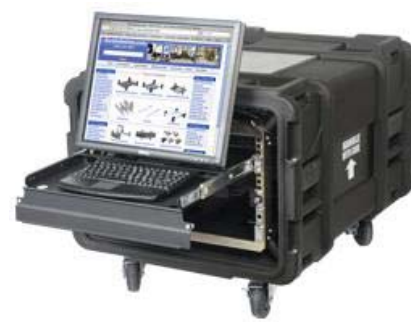
Figure 7 | Ruggedized Laptop configuration for rack case
